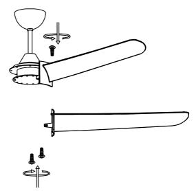
Install the blades Lock each blade on the iron plate in sequence
