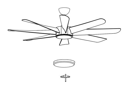
1.Screw the lamp cover on the light pan and install it
